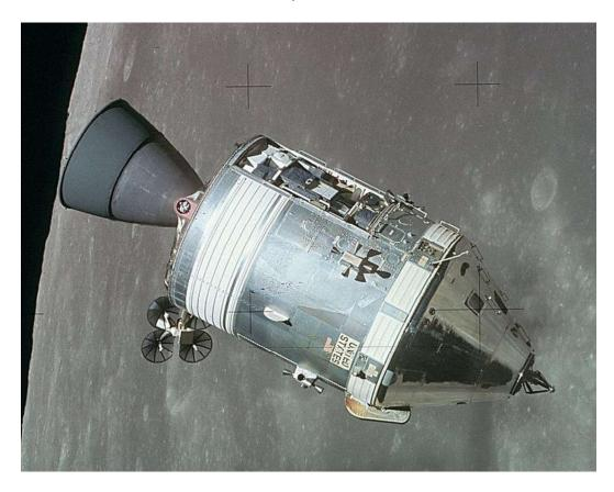
On Each "J" Mission, Two "SIM Bay" Film Canisters Were Retrieved by the Command Module Pilot, via Space Walk, During the "Trans-Earth Coast," on Day # 2 of the Return to Earth
